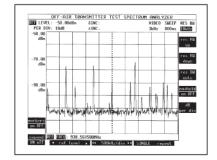
The update rate is remarkable for this type of product, allowing realtime measurements on off-air signals.
